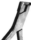
Micro Distal end cutter 13 cm / 5" 786-2106 Box Joint 786-2107 Screw Joint 786-2108 L-Key Joint With safety hold, cuts arch wires. Cuts rectangular wire up to 0.56x0.71mm, round wire up to 0.51mm and twisted wire up to 0.41mm
